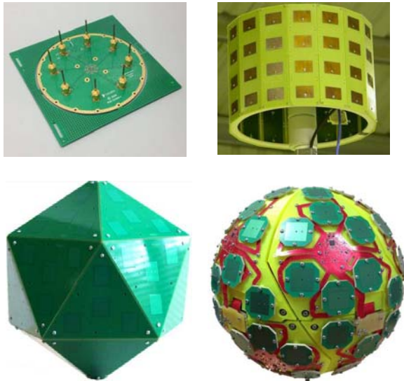
Figure 5. The proto types and current production of Locata beam-forming VRay antenna: first prototype, second prototype, third prototype and production version (from left to right, top to bottom)
