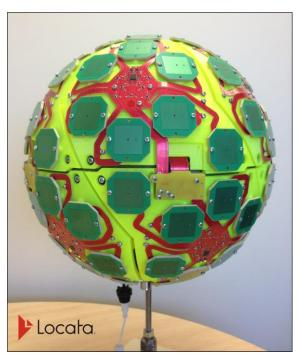
**Locata VRAY Orb-80 Antenna:** The first commercial VRAY antenna, designed to mitigate multipath for difficult machine automation applications in warehousing, supply-chain, port and industrial environments. This design will be modified by AFIT for use with GPS receivers.
