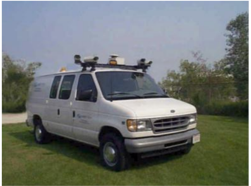
Figure 3 An example of a mounted mobile geo-referenced image capture device
