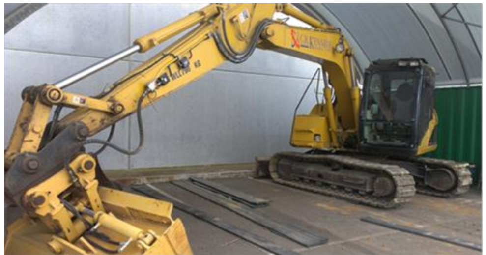
Figure 4 3D Machine Guidance system setup on excavator
