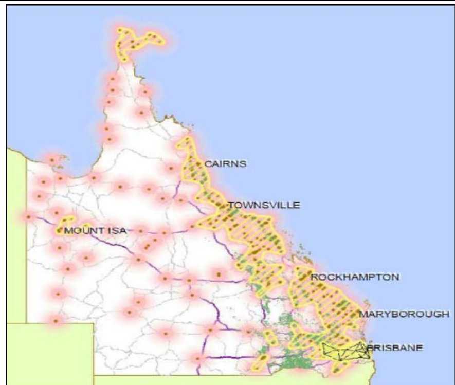
Figure 2 Shaded areas represent CORS coverage (less than 70km between stations) to support ROAMES positioning requirements
