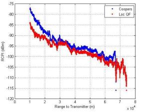
Figure 6 : Tracking Range to a LocataLite transmitting 10 watts per signal
