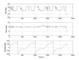
Figure 10 Aircraft roll, pitch and heading for racetrack profile at 25,000 feet on October 30
