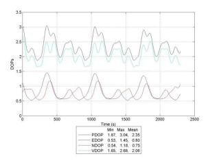
Figure 13 Dilution of precision for the racetrack profile at 25,000 feet on October 30.
