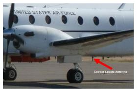
Figure 7 Antenna Mounted on C-12J
