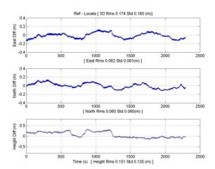
Figure 14 Difference between USAF and Locata carrier solution for the racetrack profile at 25,000 feet on 30 October.
