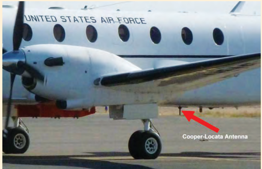
Antenna Mounted on C-12J
